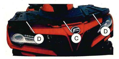
Remove battery compartment cover (C) and trunk linings (D).
