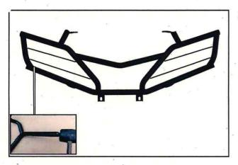
Use a rubber hammer to install the plugs (6) into the front bumper (2).
