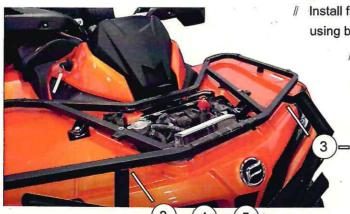
Install front bumper with upper attachment points as shown in Figure, using bolts (3), and washers (3). (4).
