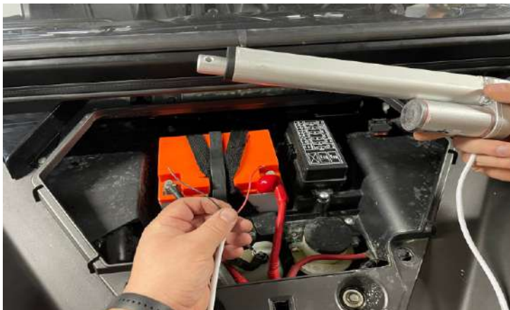
Apply voltage to the contacts of the linear actuator. Fully compress. The actuator will turn off automatically.
