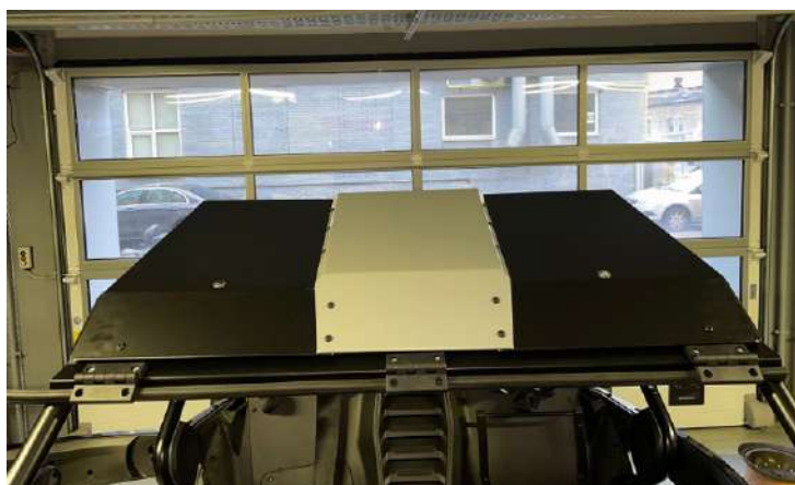
Install the aluminum roof on the frame.
