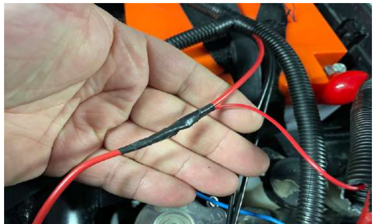
Connect the windshield wiring to the wiper wiring. Isolate the connection place.
