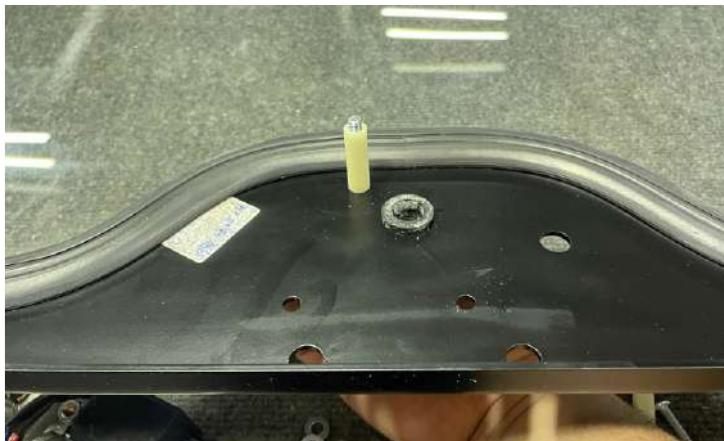
The position of the wiper motor attachment to the frame.
