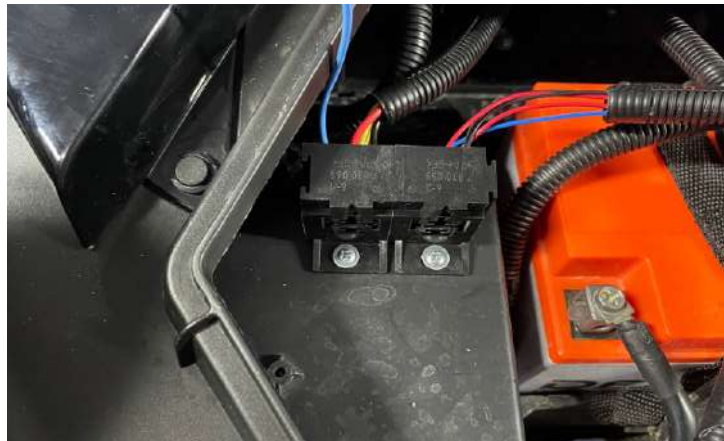
Fix the relay socket on the plastic panel.
