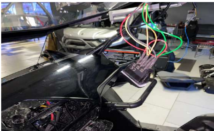
Connect the toggle switch to the electrical wiring. Install the toggle switch on the button panel under the roof.
