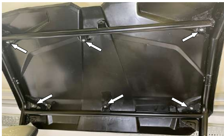
Remove the standard plastic roof.
