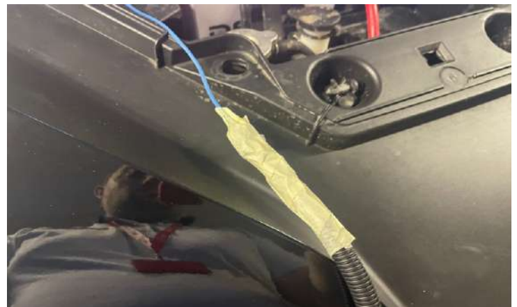
Connect the blue wire and the electric wiring of the wiper (motor connection connector).
