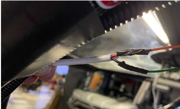
Connect the wiring of the actuator and the electrical wiring of the windshield. Isolate the connection.
