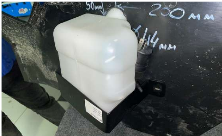
Install the washer tank by attaching it against the driver's panel as shown in the photo.
