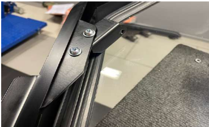
Install the left bracket of the linear actuator
