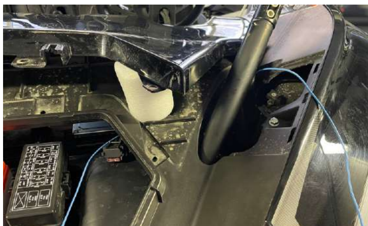
Stretch the conductor wire (a piece of blue wire) for the washer tube. The same with the right side.
