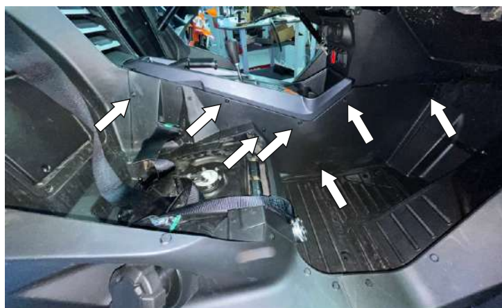
Remove the fasteners of the side panel (passenger side).
