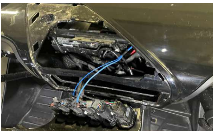
Remove the wires through the button panel in the dashboard.
