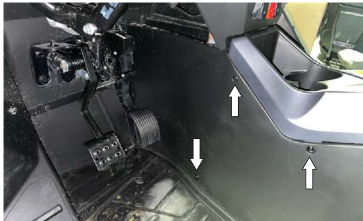
Remove the fasteners of the side panel (driver side).
