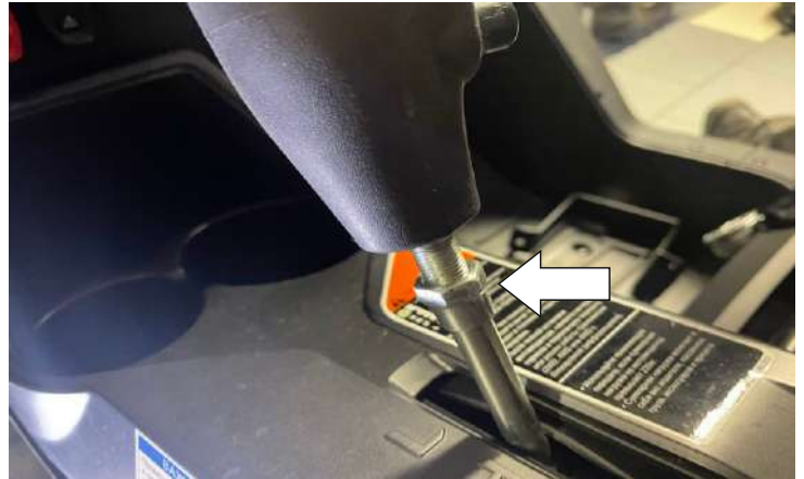
Loosen the lock nut. Unscrew the gearshift knob.
