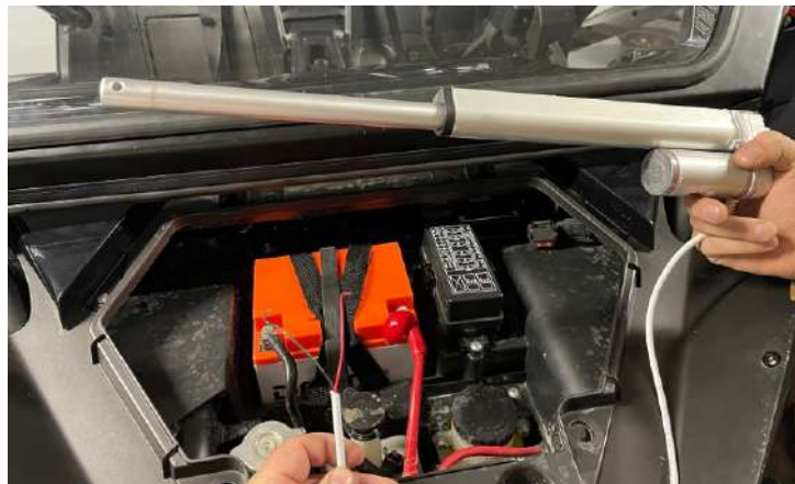
Apply voltage to the opposite contacts of the linear actuator. Fully unclench, will turn off automatically.
