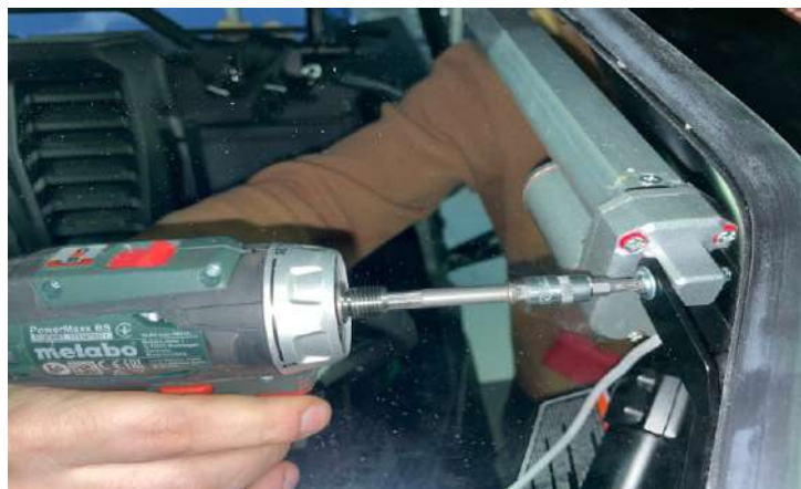
Fasten the linear actuator.
