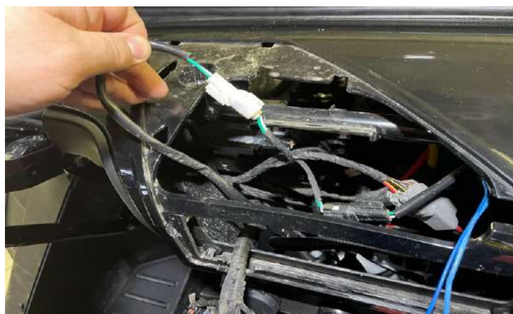
Take the standard cigarette lighter connector through the button panel in the dashboard.
