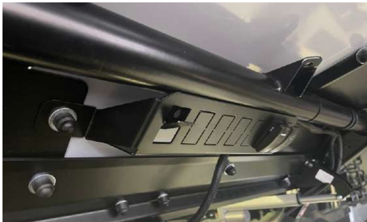
Remove the cap of one button in the panel under the roof.
