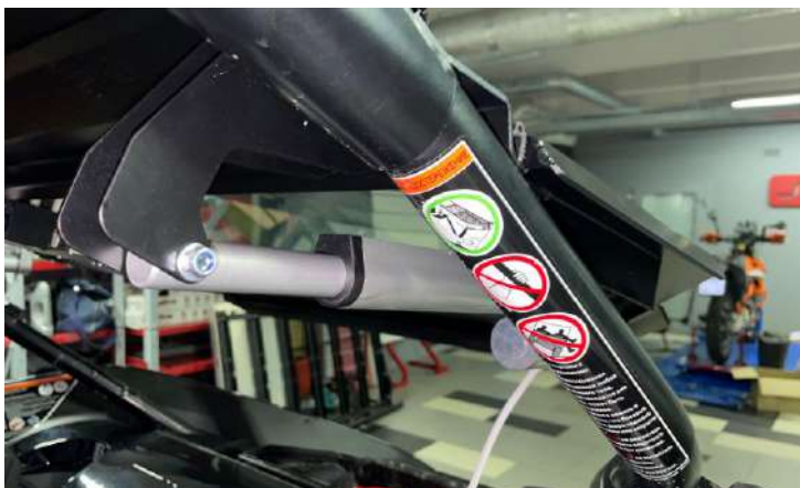
Install a linear actuator.
