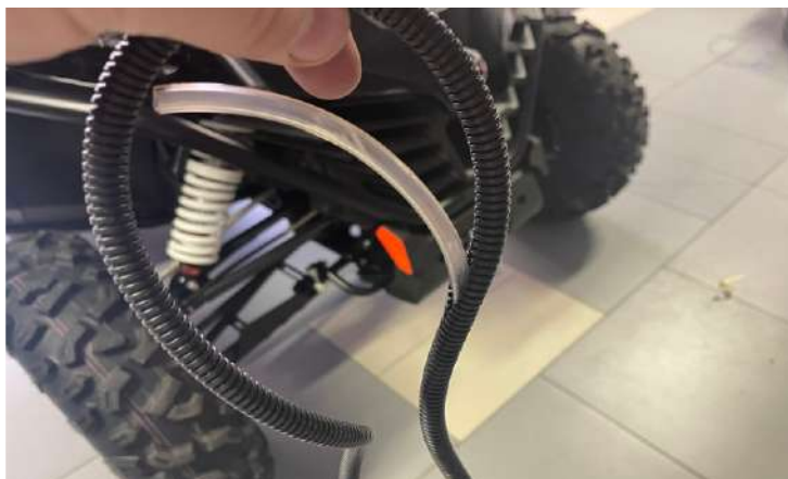
Thread the washer pipe into the corrugated tube.
