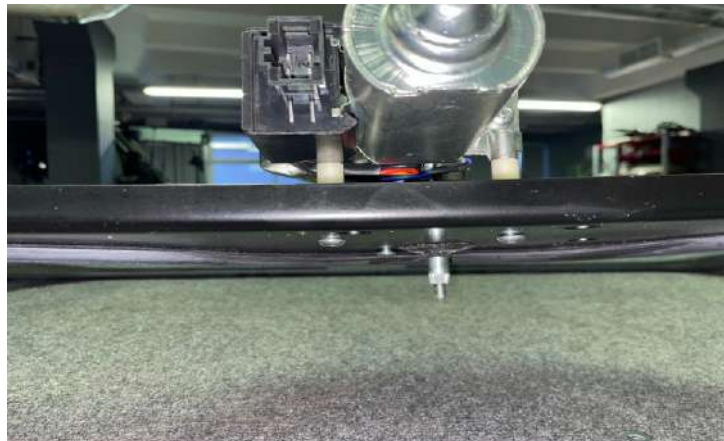
Fasten the wiper motor.
