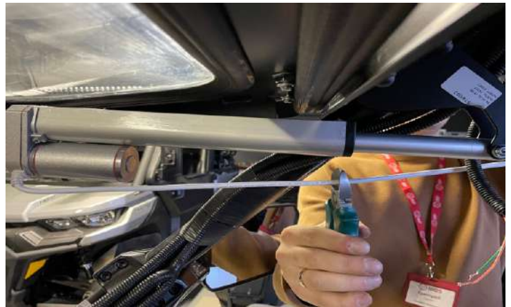
Cut off part of the wiring of the linear actuator, as shown in the picture.
