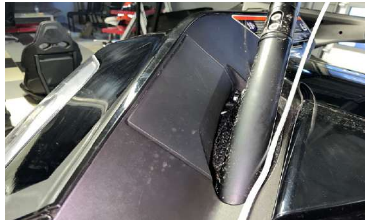
Remove the button panel aflat, with a little effort towards the back part.
