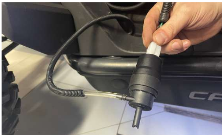
Install the washer tube and the connector to the water pump.
