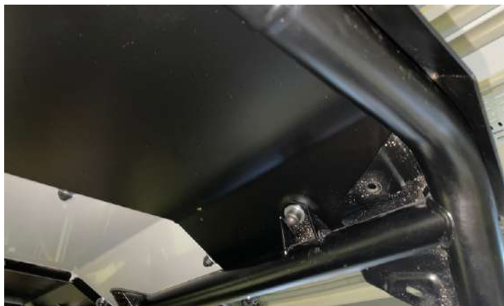
Set roof fasteners to the back of the frame.
