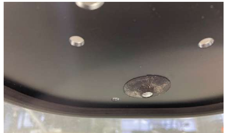
Install the wiper motor seal.
