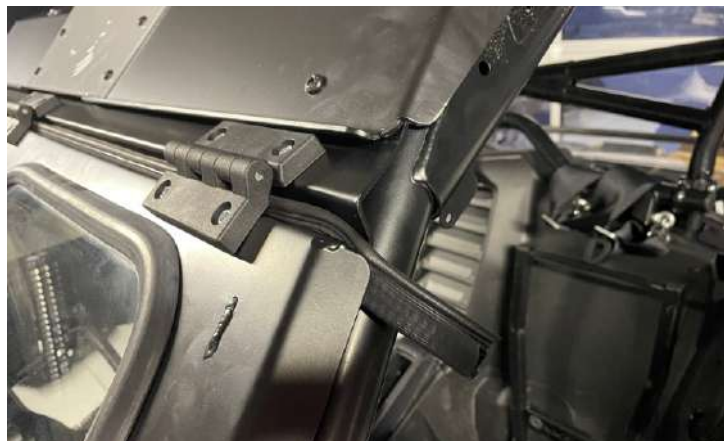
Gradually tighten the fasteners of the brackets, lifting and lowering the frame (the brackets align with each other).
