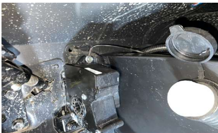
Connect the negative terminal (black) to the pedal bracket as shown in the picture.
