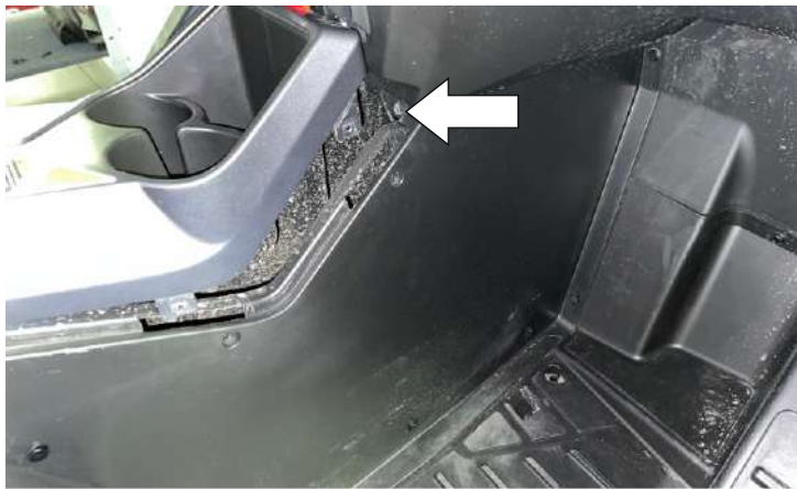
Unscrew the bolt from right part of central panel.
