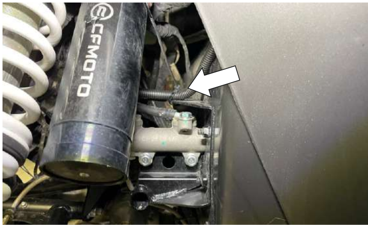
Fix the electrical wiring of the windshield to the frame in the left front arch.
