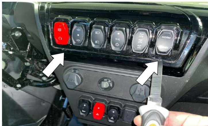
Use a puller to detach the central panel with buttons (below).
