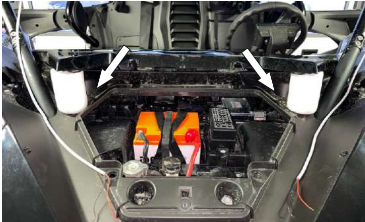
Unscrew the panel bolts (pointed in the photo). Slightly lift the panel. Put spacers from the frame (windshield).
