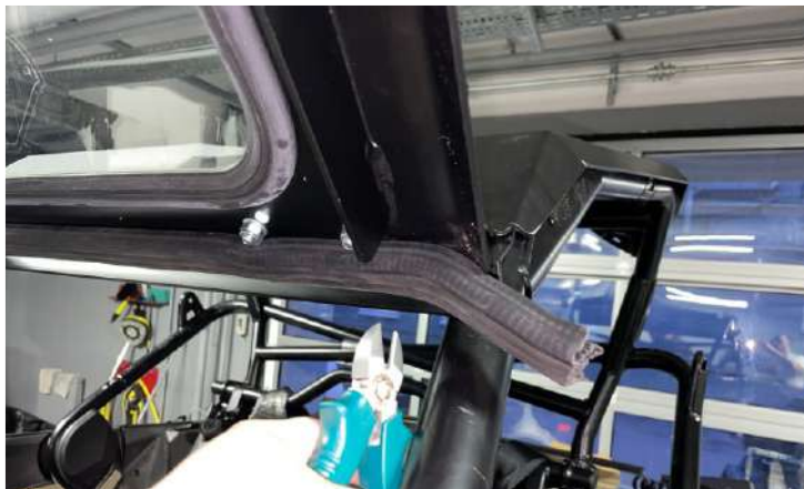
Install the sealing gasket on the frame as shown. Cut off the excess.
