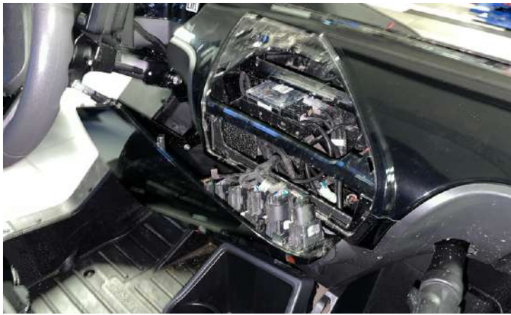
Remove the button panel horizontally, with a little effort towards the back.
