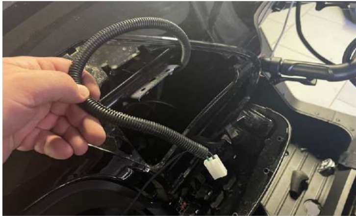
Pull the end of the electrical wiring through the dashboard - down to the washer tank.
