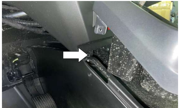
Unscrew the bolt from left part of central panel.
