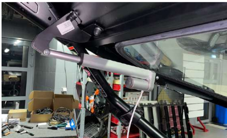
Linear actuator on the driver's side.
