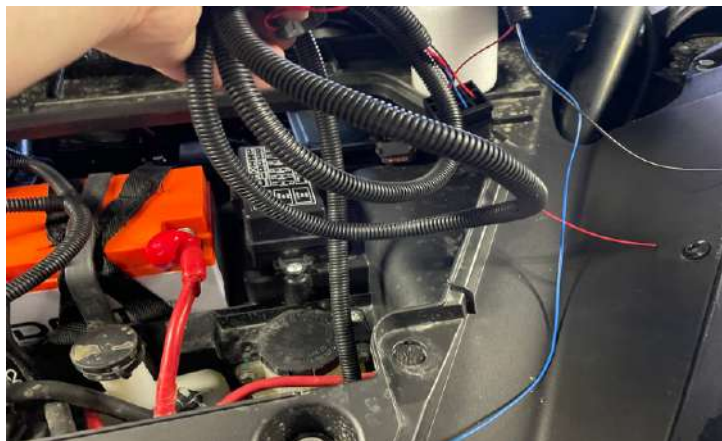
Place the wires in the engine compartment. Pull off excess wires with a plastic clamp.
