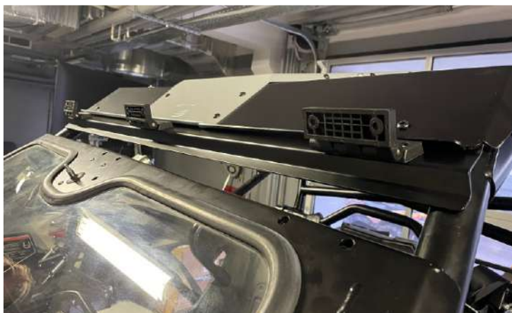
Attach the windshield to the frame.
