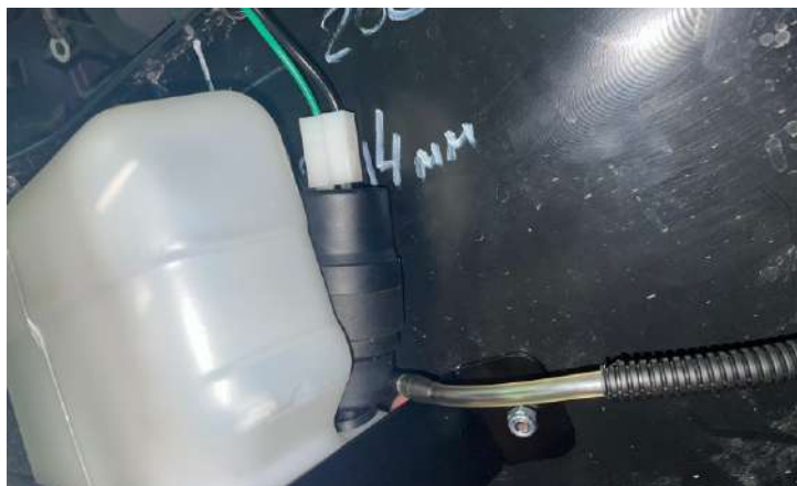
Install the water pump in the tank. Install the plastic panel of the driver's side.
