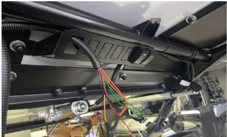
Pull the end of the electrical wiring through the panel.
