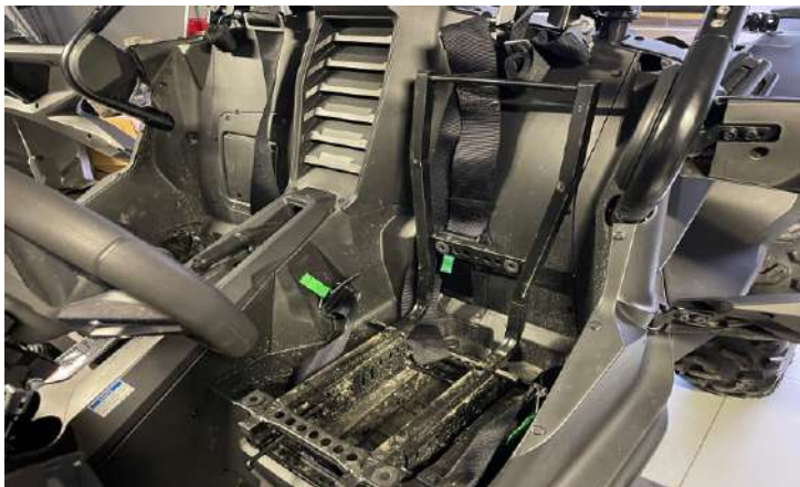
Remove the frame of the driver's seat.
