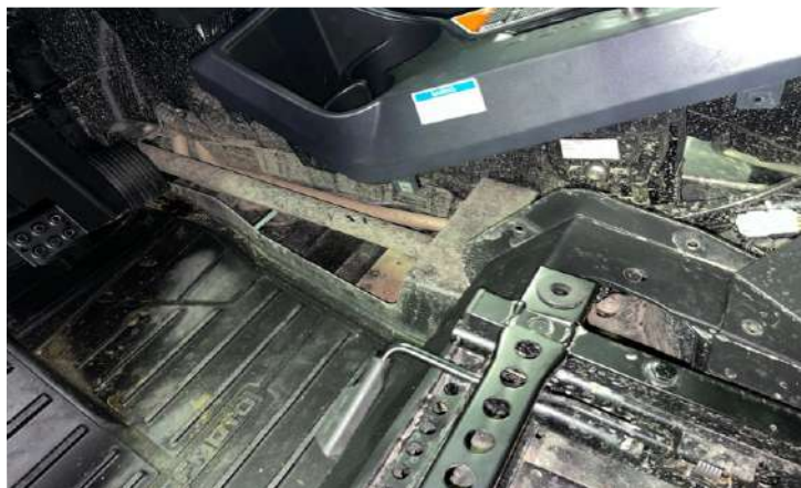
Remove the driver's panel.
