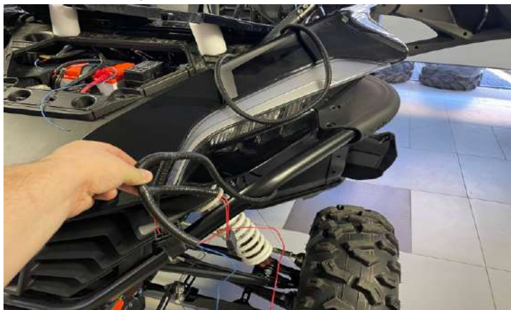
Stretch the electrical wiring of the windshield from the button panel under the roof to the engine compartment.
