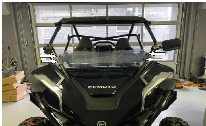
Remove the standard plastic glass.
