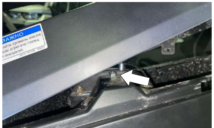
Unscrew the driver panel mounting bolt.
