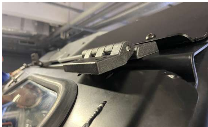
Align the brackets with the windshield.
