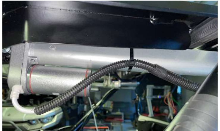
Put the wires in the corrugated tube. Attach to the linear actuator.
