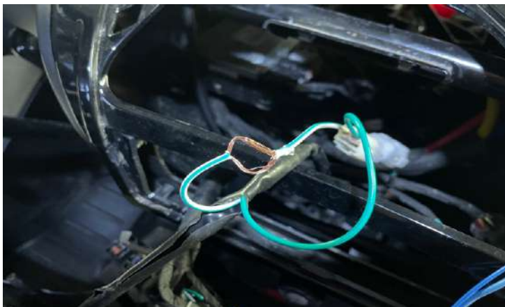
Clean the insulation from the green-white wire and attach the two blue wires. Isolate the connection.
