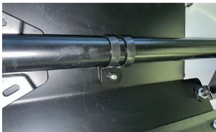
Set the roof fasteners and clamps.
