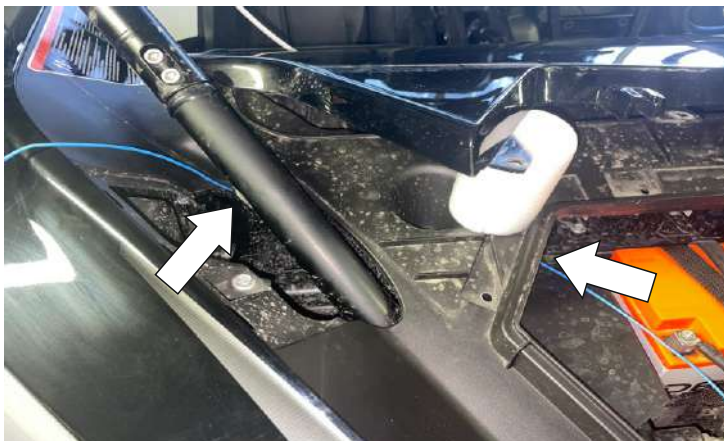
Stretch the blue wire (remainder) as shown in the photo. Use it as a conductor.
