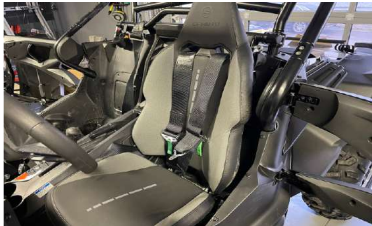
Remove the driver's seat.
