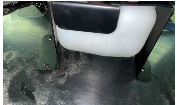
Mark the mounting points of the bracket on the plastic. Drill 7-8mm holes in the plastic.
