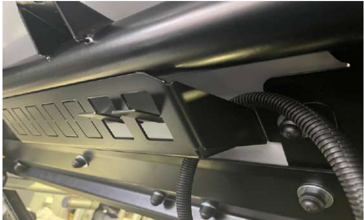
Remove the caps of 2 buttons in the panel under the roof.
