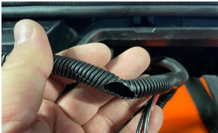
Make an incision in the corrugations of both electrical wires to output the blue wires (ignition connection).
